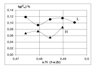
Fig. 3- Mechanical tangent of losses versus x.
