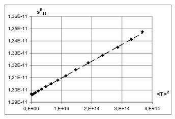
Fig. 6- Non-linear compliance increase versus quadratic mean stress.
