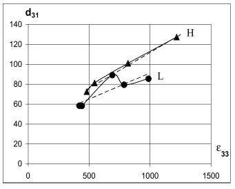
Fig. 4- Piezoelectric d<sub>31</sub> coefficient versus dielectric constant.
