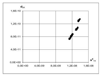
Fig. 7- Piezoelectric  $d_{_{31}}$  versus compliance  $s^{E}_{_{11}}$ .
